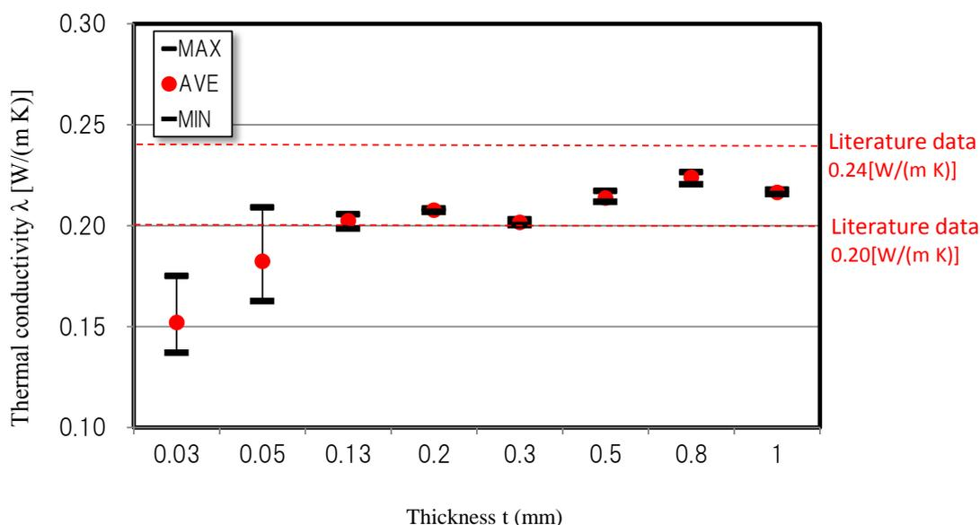
Fig. 1 Thickness and thermal conductivity of PTFE sheet
