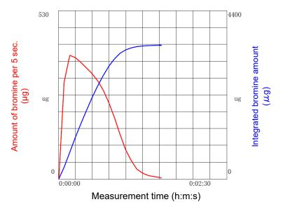
Table 1 Result of measurement of bromine index (one-component inner burette)
